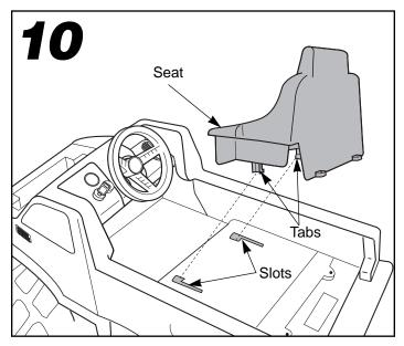
• Insert the two tabs on the bottom of the seat into the slots in the vehicle body.
